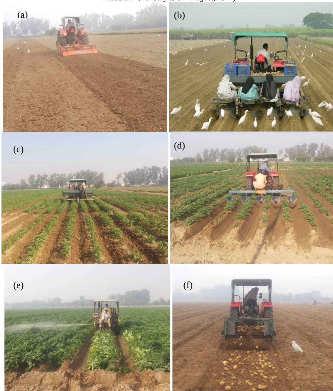
Fig. 1. (a) Field preparation using rotavator, (b) Planting operation with semi-automatic planter, (c) Interculture operation (weeder cum fertilizer applicator), (d) Ridging, (e) Spraying of chemical with gun sprayer and (f) Potato digger cum elevator.
