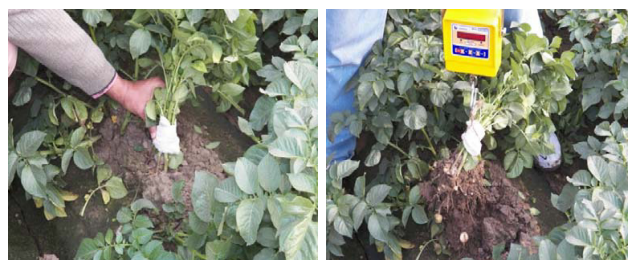
Fig. 5: Estimation of root pulling force through dynamometers
