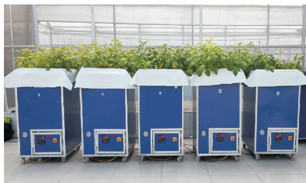
Fig. 8: Portable aeroponic systems installed at CPRS Jalandhar
