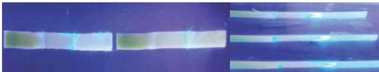
Fig. 7. Lateral flow immunoassay to analyze the conjugation of PVX Ab-QD visualized under UV transilluminator
