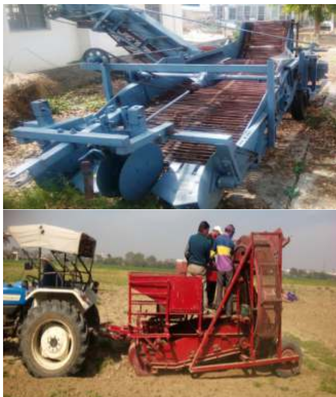
Fig. 19. Tractor operated potato combine harvester (Prototype I and II)
